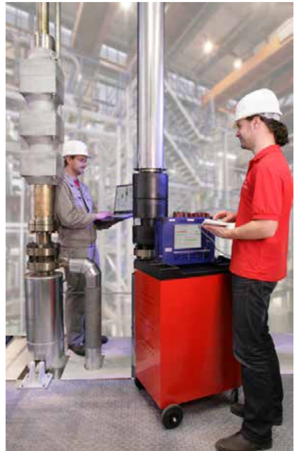
Set-up for CRDM factory acceptance test
