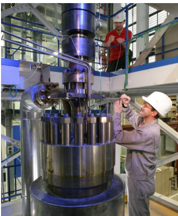
Instrumentation of CRDM during qualification test
