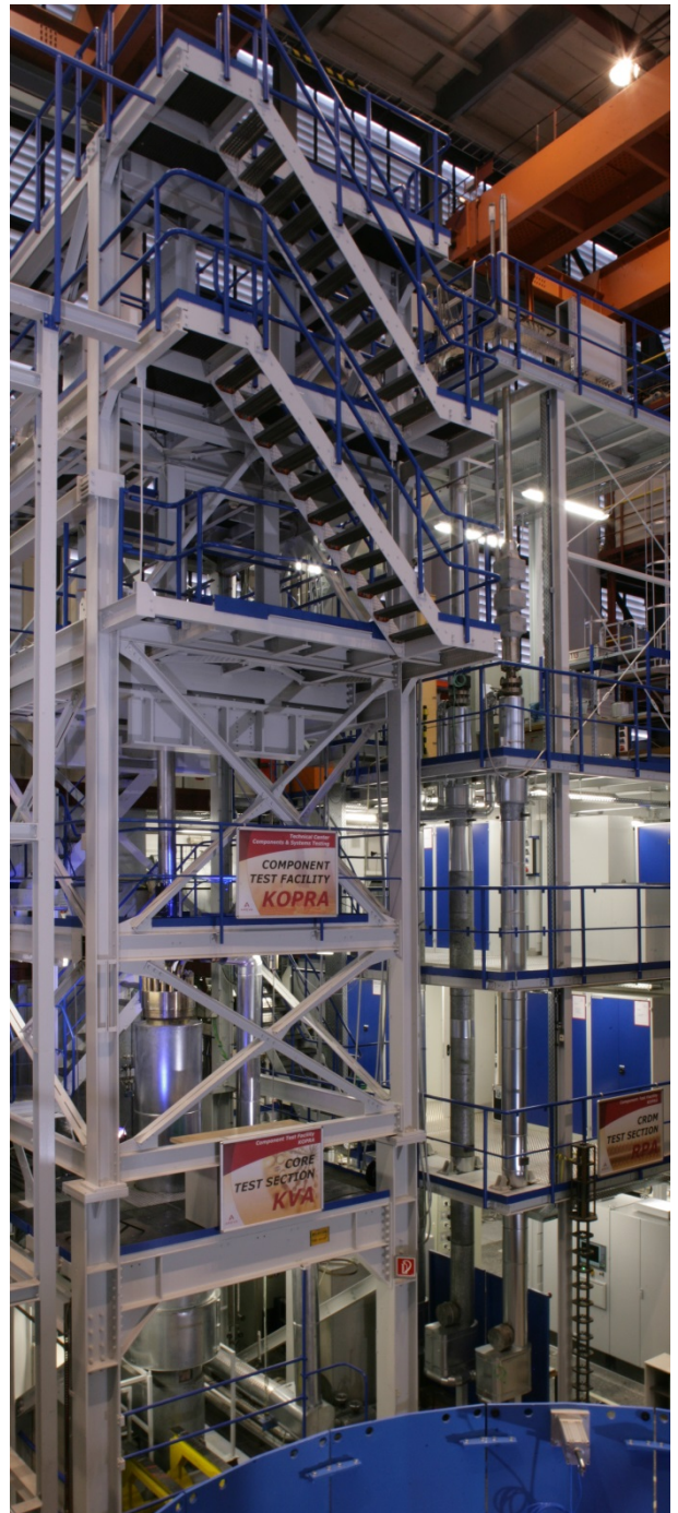
Test set-up CRDM qualification for EPR™
