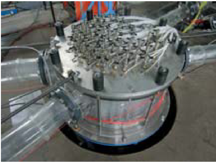
EPR™ reactor pressure vessel mock-up: Romeo
