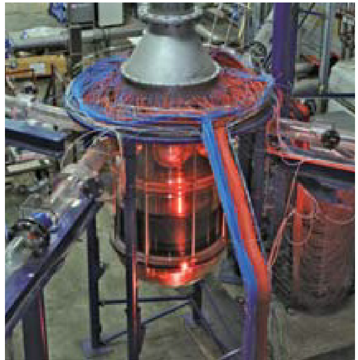
EPR™ reactor pressure vessel mock-up: Juliette
