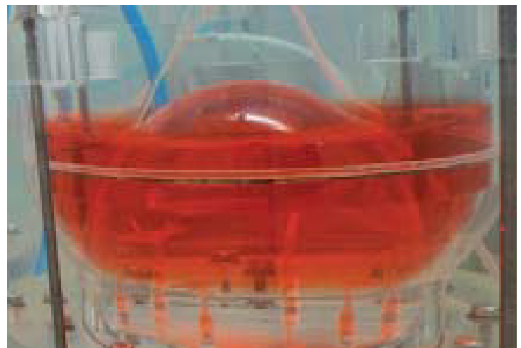
Gas-liquid interface in a tank under micro-gravity conditions
