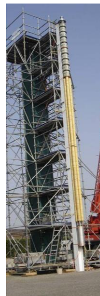
Electromagnetic pump drainage tool in the manufacturing process, which is introduced into the reactor, and is integrated in an automatic instrumentation and control system
