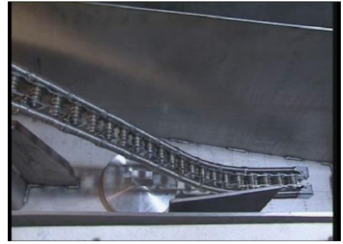
Flexible drainage end-piece for an electromagnetic pump
