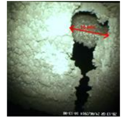
Remote visual inspection of the heat baffle in the SPX reactor (DEM) – Views of baffle access and the inside of the baffle with solidified sodium drops
