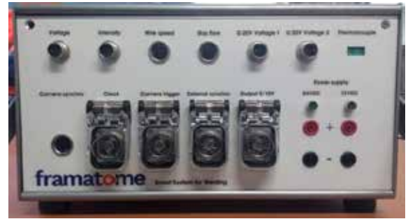
Standard SSW device configuration, front view
