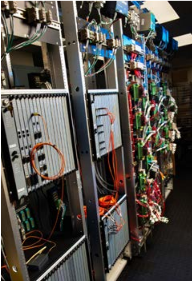
1E Tricon System shown in the I&C test lab at Framatome's Lynchburg, Virginia, Operational Center of Excellence
