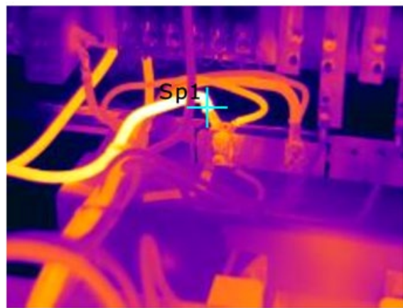
Example of Infrared thermography analysis, performed on a safety inverter
