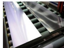
Z4B-BQ fuel channels are fabricated with established rolling and forming processes
