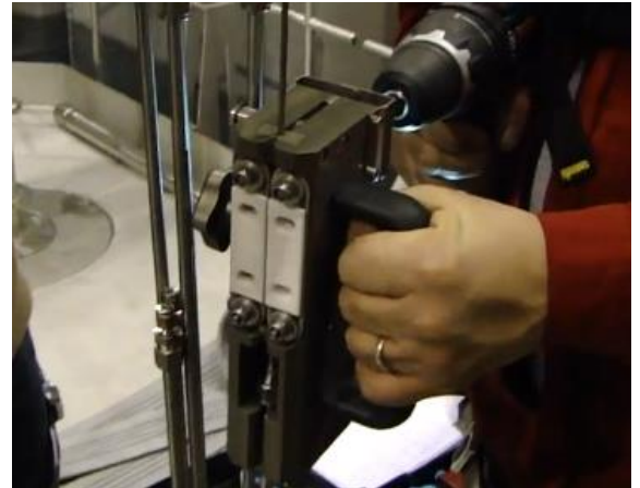
TC continuous insertion tool demonstration on a reactor mock-up
