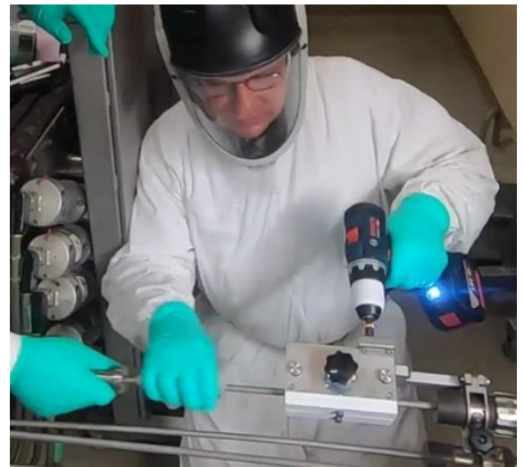
Semi-automatic continuous thimble tube withdrawal and insertion tool
