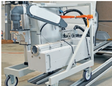
Loading of the mobile ultrasonic inspection system
