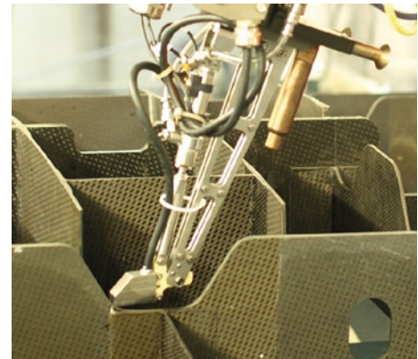
Custom made compact UT probe for inner-radii testing of CFRP structure
