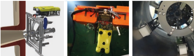
FRANIS – CAD model, Framatome training center, telescopic arm for UT probes bearing
