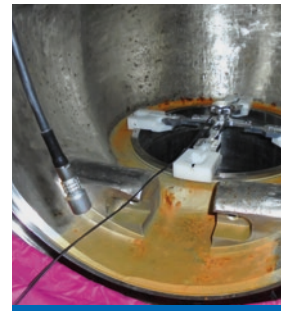
ET probes holder in examination position
