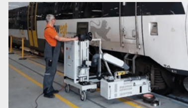
Mobile in-maintenance PAUT of assembled train axles in railway industry
