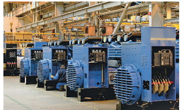
Genset assembly in supplier facility
