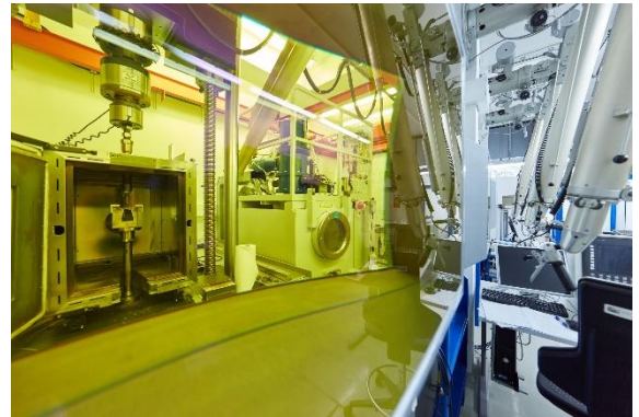
Single-edge-bend bar testing device in the hot cells
