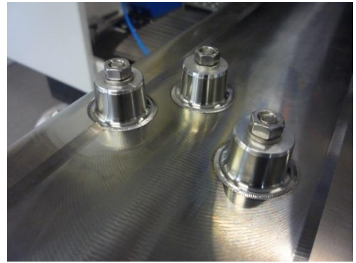
Welding example (Zircaloy material)
