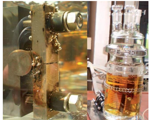
Crack initiating attempt at notched bend test specimen under medium conditions
