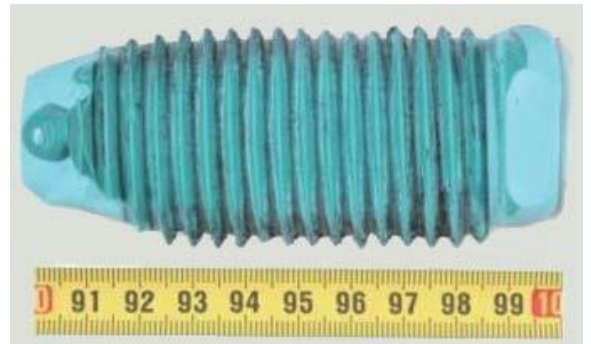
Replica of a large bore thread out of a ductile cast iron housing for further thread profile measurements
