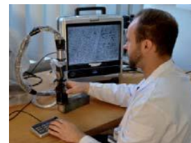
Direct grain structure evaluation up to X1000 with digital microscope
