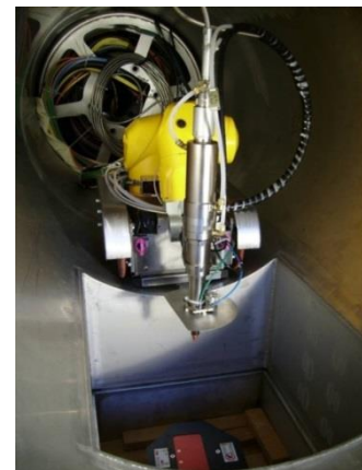
Laser cutting robot successfully used at Super-Phenix
