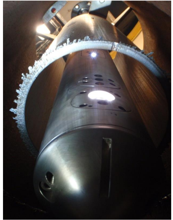
Inspection and orbital laser cutting rod able to cut tubes and plates up to a distance of one meter
